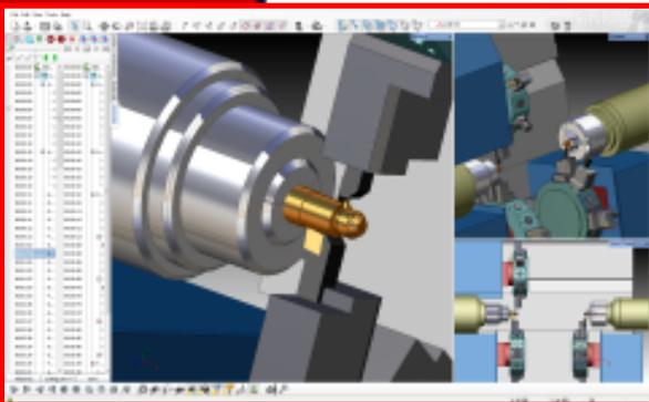
**SprutCAM** can create NC programs for the synchronised control of multiple machine axes (spindles / turrets). In SprutCAM it is possible to insert synchronisation points between operations as well as between the commands inside an operation. This unique feature allows a substantially boost in machine output by avoiding time consuming machine program 'prove-outs' whilst also allowing the most efficient and safe (synchronised) use of the available machine axes.
