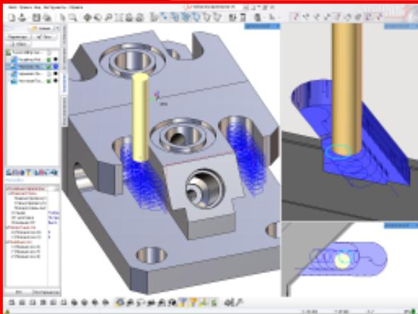
**SprutCAM** milling strategies include features for creating 'High-Speed' milling tool paths. Trochoidal 'penetration' tool paths, **smoothing of sharp corners, arc approach and retraction** all help to ensure smooth tool paths and a consistent area of cut, which, together with the calculated lead in / out moves enables the use of high speed milling.
